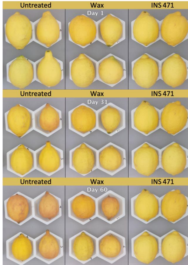
Figure 2: Time-lapse images of INS 471 treated lemons compared against untreated lemons and lemons treated with conventional wax.
